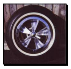
Hurst wheels were produced from early 1965 to mid 1969 by George Hurst. They were constructed using a forged steel rim with aircraft grade aluminum center spokes. The removeable chrome trim ring, center cap, and special lug nuts made these wheels quite attractive. Each wheel was serial numbered and had a lifetime guarantee.
